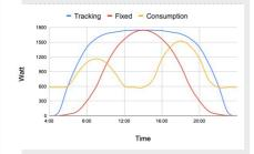
This graphic demonstrates why tracking (blue line) gives you a serious output boost in comparison with a static roof system (red line). The yellow line shows the typical household usage when people go out to work etc.
