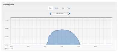
This is an image of the production curve from the PV-4 at our HQ on 24th January which perfectly demonstrates the fact that the tracker is following the sun!
